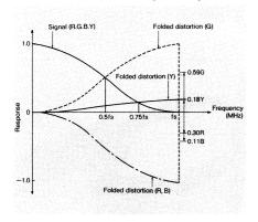
reduce moire, the FP-C1 employs an optimized quartz filter. The spatial offset technology for higher resolution also contributes to reduction of moire.
